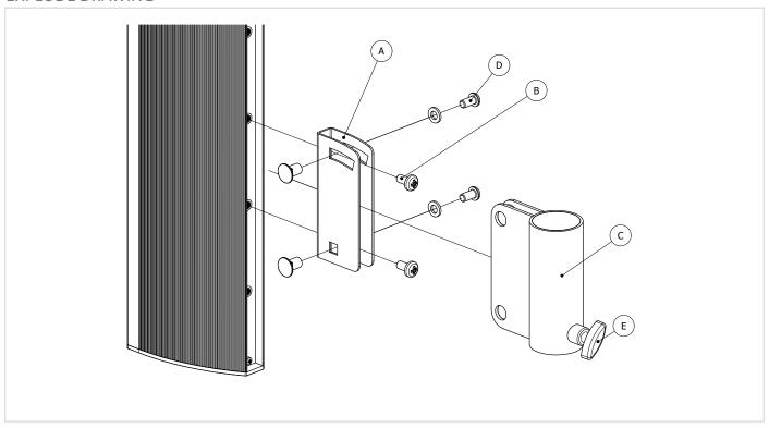
Install the speaker part ('A' - which is standard included with the KYRA6/12 series loudspeakers) at the provided location on the rear side of the loudspeaker.
